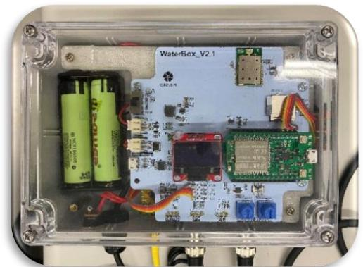
Figure 2: WaterBox setup with replaceable batteries
